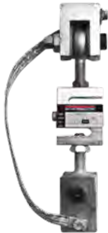
Module with RL20000 s-beam load cell.
